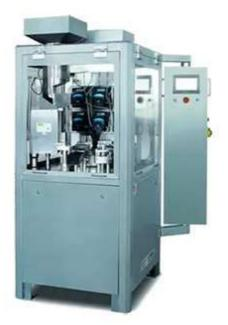
This machine is a hard capsule filing machine with intermittent liquid injection pump control system. It meets GMP requirements and has advantages like compact structure, smaller size, low noise, accurate filing dosage, complete functions and smooth operation. The machine can complete the whole functions from capsule feeding, separating, filing, rejection, locking, until finished product discharging.
