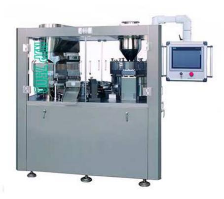
The design is precise and beautiful, and the operation is stable and reliable. It can automatically complete a variety of procedures such as seeding, splitting, filling, rejection of waste capsules, locking of capsules and export of finished products. Fully enclosed 12-station turntable, the module is designed in three rows of 54 holes, this model is a special equipment for the production of large-capacity hard capsule filling.
