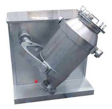
Three-dimensional mixer Drug powder mixer The multi-dimensional mixer base is made of model steel and is covered with stainless steel. The structure of the machine base is reasonable, which can effectively stabilize the whole machine and fully meet the requirements of GMP for medicines.
