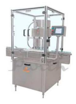
Automatic VIAL Cap Sealing Machine is versatile, self-supported on stainless steel leg with height adjustable adjustment system. This vial capping machine is precision built on sturdy welded MS frame completely enclose in stainless steel sheet and doors are providing to facilitate the servicing of machine.
