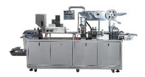
DPP-250 Blister Packing Machine is widely used for packing tablets, capsules, candy, chew gum and other similar shape solid articles with alu-plastics & alu-alu blister in the pharmaceutical, chemical, foodstuff industries. The machine can finish the following actions automatically: Aluminium foil or Plastic (PVC) blister forming, automatic material feeding, PTP alu-foil press and heat-sealing, press the batch number & perforation and punching.
