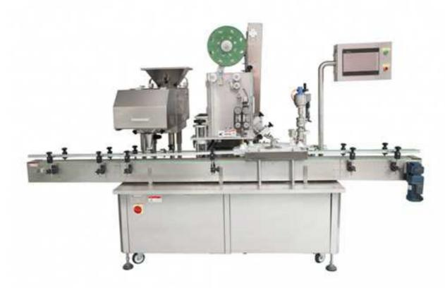
3 in 1 Capsule counting and packing machine is an innovation design multi-function compact package system, which is consists of 8 channel counter, desiccant pouch insert and rotary capper with cap feeding elevator. It is ideal packing machine for lab and space limited customer. The machine handles a wide variety of tablets, caplets and both hard and soft capsules with different shapes and sizes bottle and cap.
