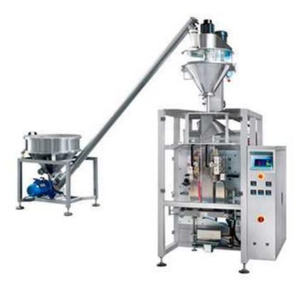
Powder pouch packing machine is fully automatic powder dosing and bag making machine, applied to dose target weight of dry powder and fill into different size of pillow bag. It loaded with a continuous flat roll of film with artwork. The powder pouch packing machine make bag from the film and simultaneously fill the bag with powder product and seal it.
