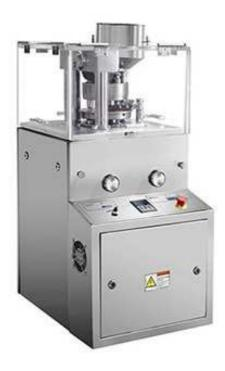
Rotary Tablet Press With 9 Punches is a new generation product by our factory, and this machine is a single Roller continuous automatic tablet press for pressing various kinds of different shape tablets and plain tablets It is mainly used in pharmaceutical industry and also the chemical, food, electronic industries.
