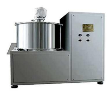
This machine makes damp granule into beautiful pellet by setting rotating centrifugal disk, lower, and pneumatic nozzle. Feed damp granule into rotating centrifugal disk, start fan then start rotating centrifugal disk. It can make the damp granule in float and circle by the air from gap, rotating centrifugal strength and itself gravity, appear circle rope-turning movement and become high-degree ball shape pellet.
