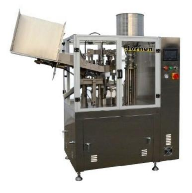
NF80A Automatic Tube Fillers are designed and engineered to produce outstanding quality and precision tube filling and sealing of, plastic, metal plastic laminate, and aluminum laminate tubes with the output up to 80 tubes per minute. This machine is widely used in pharmaceutical, food, household chemical and cosmetic, etc., industries.
