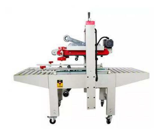
This carton sealer is mainly used for household electric appliances, textile, foods, general merchandise, medical, chemical etc. Industries to seal and packcartons in the way of by-itself or being fitted with the production lines. Adhensive bands are used to seal cartons with the ability to do both up and down sealings in one time, economical, fast and easy toregulate. The product packed in can be made much more impressed with the word-printed band used.
