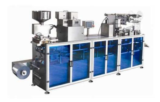
This machine can continually and automatically complete the packing proceedings, is blister cap form-taking, medicine-feeding, heat sealing, printing lot no, and cutting into format. It Has advantage as compact structure, full function, gear wheel working, and accurate Synchronization, stable cooperation, easy to replace the mould, low cost and needn't to equip Auxiliary unit. Turn on power and connect it with cooling water, you can produce in a large scale.
