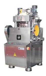
This machine is designed for pressing all kinds of granular materials into a round plate, and is suitable for batch production of the basic equipment. Rotary speed, the depth of the filling and tablet thickness can be adjusted. The mechanical buffer device can avoid the overload and cause damage to the machine. The machine can be another match suction powder box, through the suckers to absorb dust, avoid bonding jams, and recycle raw materials to use.
