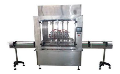
The machine is an automatic liquid filling device which is composed of PLC, human-computer interface, and optoelectronic sensor and air-powered. The machine adopts time control theory, switch time of the solenoid valve and metering pump to control the filling dose precisely. The machine is unique in simple operating, stable performance, accuracy measuring, no dripping or leaking and convenient in changing model.
