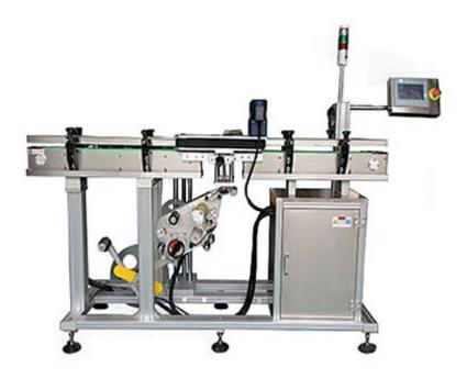
This machine is labeling on product bottom surface, machine conveyor with two parts, also with the clamping device to fix product not fall when labeling on the bottom.
