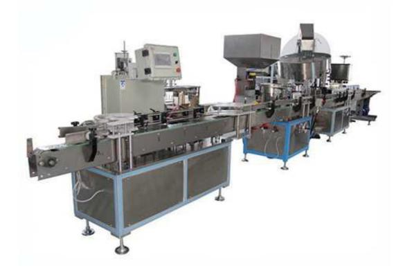
CJXH-2800B automatic aerosol filling machine consist of can arrange machine, rotary liquid filling machine, valve insert machine, rotary sealing and gas filling, automatic weight checker, water bath, nozzle presser, cap presser, ink jet printer, carton sealing & strapping machine.
