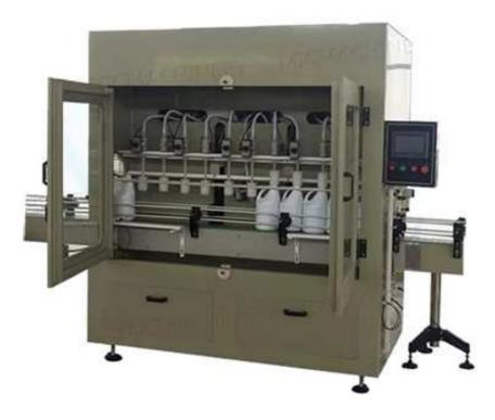
This filling machine is suitable for: pesticides, chemicals, bottled agent type liquid dispensing, bottle filling, Applicable to a variety of different types of containers.
