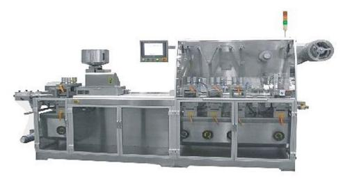
This machine is suitable for sealed blister packing of wide range of specifications of capsule, tablet, syringes, ampoule, medical appliances, food, electron device, and small hardware device which is used in pharmacy, Medicine Apparatus, food, electronic, small hardware etc.
