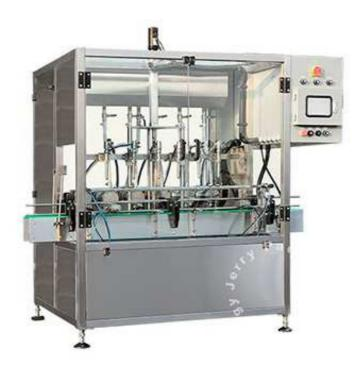
This series of filling machine adopts gear pump flow meter filling method. This machine adopts PLC control, servo control, and quick filling after quick loading, which can ensure the fastest filling speed and prevent filling. The process is overburdened, and the pneumatically closed filling nozzle can effectively prevent dripping during the filling process. This machine is easy to operate and debug, and is widely used for quantitative filling of various oils and other liquid products.
