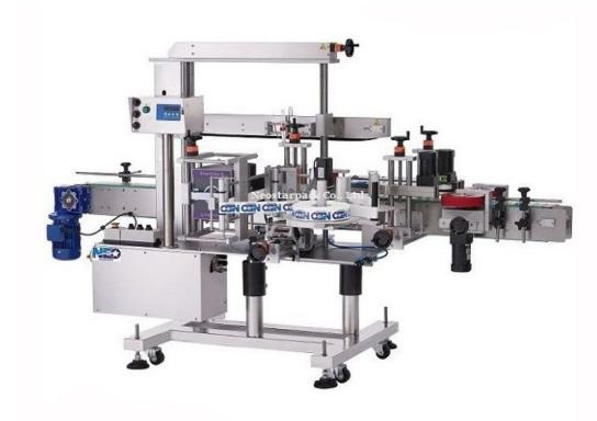
Automatic Front and Back Labeling NLD-300 is suitable for all kinds of bottle. Such as oval shaped, square, flat, and round bottles. It can use both label applicators simultaneously or run individually.
