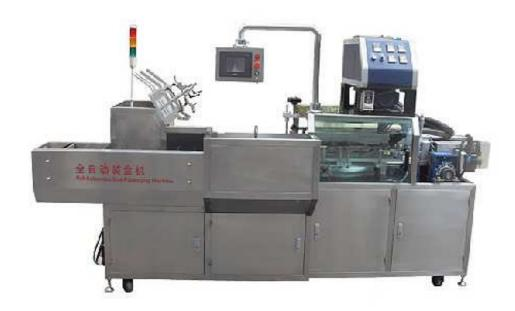
Full automatic box sealing machine is more intelligent than semi box sealing machine. It realizes box opening, product filling, box gluing and box sticking full automatically.
