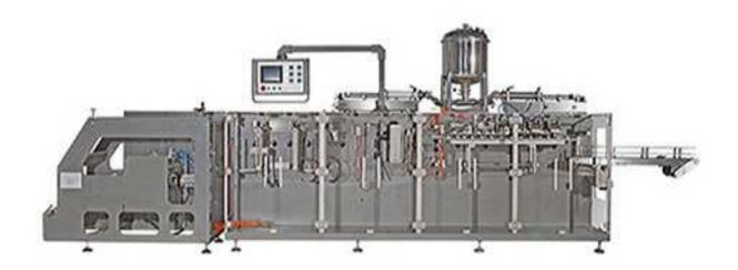
It is designed for stand up pouch (doypack) with zipper (zip lock). With different type of dosing system, such as screw auger filler, volumetric cup filler, multi-head filler, the machine can be used to pack powder, liquid and granule product, such as sugar, spices, juice, tomato paste, nuts, candy, washing detergent, lotion, pills, capsule, pesticide, fungicide, etc.
