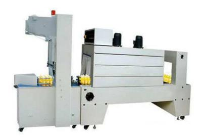
The bottle shrink packaging machine include two parts: semi-auto sleeve wrapper and PE film shrink wrapping machine.
