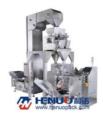
This machine is specially designed for packaging all kinds of granules, such as sugar, salt, seeds, coffee beans, rice, dried fruits, candies, pills, etc., into premade pouches such as flat pouch, gusset pouch, stand up pouch, zipper pouch, doypack, etc.
