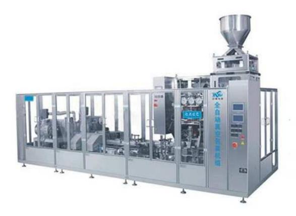
The 500N/500N2 internal suction vacuum packaging machine can realize automatic loading, weighing, bag making, filling, shaping, vacuum extraction, sealing, bag cutting and finished product transportation, and turn the bulk material packaging into a hexahedral small package with high added value. The packing is fast and stable. The unit is widely used in the vacuum packaging of grain products such as rice grains and powders such as coffee. It is suitable for mass production.
