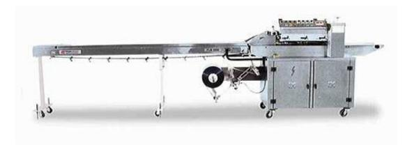
FLM 5000 is the reverse horizontal flowpack packaging machine where the bobbin of the machine is located on the bottom.
