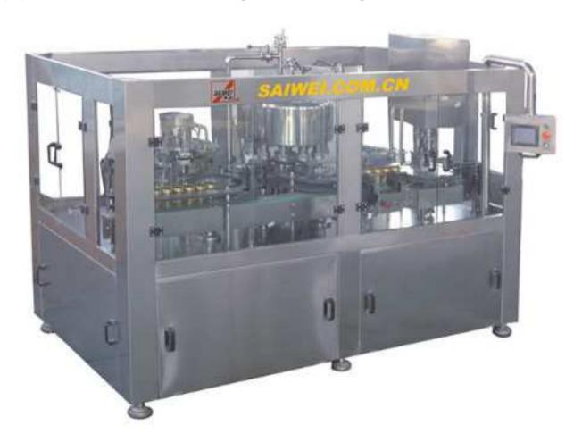
YGF series of can filling and sealing monobloc machine, whose technologies was introduced from SWEDEN, is specially applicable for washing filling & sealing non carbonated drink into can at room temperature or high temperature. Capacity of this series of machine is from 1500 to 9000 can per hour, based on 330ml can.
