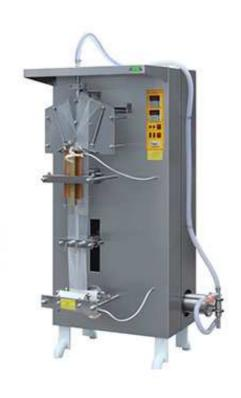
This automatic drinking water Liquid Packing Machine adopts food grade 316/304 stainless steel structure, which reaches the international health standard. This machine has stable and reliable performance, simple operation and low failure rate.
