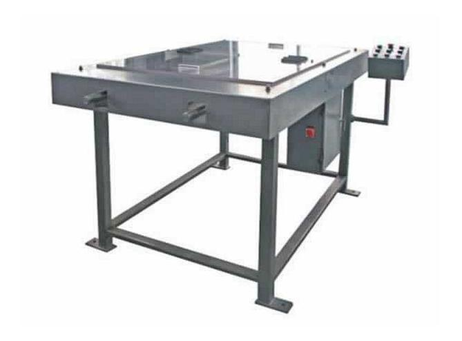
This device XP100 / 500 is used for unloading and moving the glass infusion bottles or vials of the card for the sterilization of the savings table for the container.
