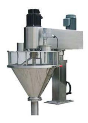
The screw measuring machine is metered by a screw feeder, that is, the cavity of the screw groove is used as a measuring container, and in each dispensing cycle, the speed of the screw rotation is controlled, and the physical quantity of each rotation is controlled, thereby Achieve the purpose of measurement.
