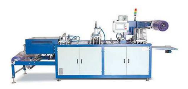
JH450A model Cup lid making machine use plate board heating system, servo motor roller the sheet. Mold is easier for change, and use small power of the machine, mold cost are small, power consumer lower. This machine mainly use to produce lid, and small trays.
