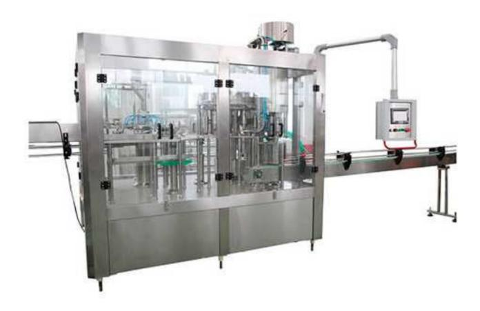
This automatic juice filling line is suitable for tea, juice and etc. The machine is 3 in 1 monoblack composed of washing, filling, capping in one unit. The riser adopts overturning device, and filling valve is special designed for hot filling. The capping head we adopt Italy technology.
