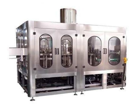
This machine is core machine in beer/carbonated drinks production line. It is for fill and seam of beer and other carbonated soft drinks (aluminum can/pet can), like cola, soda, energy drinks and so on.
