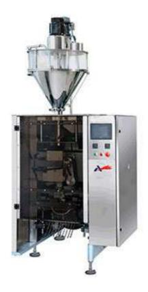
This machine is suitable for automatic packaging of powdered materials such as flour, fine sugar, milk powder, monosodium glutamate, seasonings, food additives, pesticides, washing powder etc.
