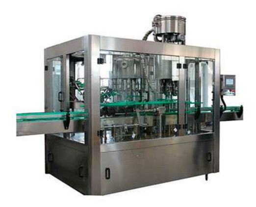
CGF is a kind of professional filling machine integrator for water filling machine. It is multifunctional which can be used for washing, filling and capping. It is a kind of advanced filling machine integrator which is innovated in following the process requirements of filling pure water, mineral water, wine, etc. based on the importing and assimilating the foreign advanced technology.
