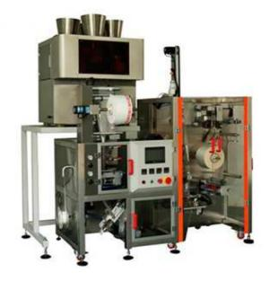
Designed for pyramid tea bag packing. Bag type is rectangular, three sides sealing. Applicable packing materials are PLA, Nylon, non-woven fabrics, etc. To operate the machine needs compressed air supply with a pressure of more than 1.2 MPa. Working capacity is 30 – 40 bags per minute.
