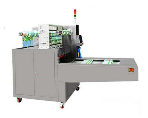
GT680 Automatic gas flushing food tray pack sealing machine also called Automatic modified atmosphere tray sealing machine.
