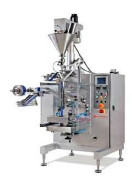
PLC control unit, servo motor controlled film transport, connection apparatus and hoses for aspirator group. Metallic grey colored and surfaces of the machine that are in contact with the product made stainless.
