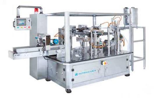
There are two systems of filling the pump piston and pump lobe. Operation of the machine with a touch screen control, with an efficient power consumption and features that really support this machine. Stainless steel cover body for main body and electric panel control. Stainless steel bar for open pouch sensor.
