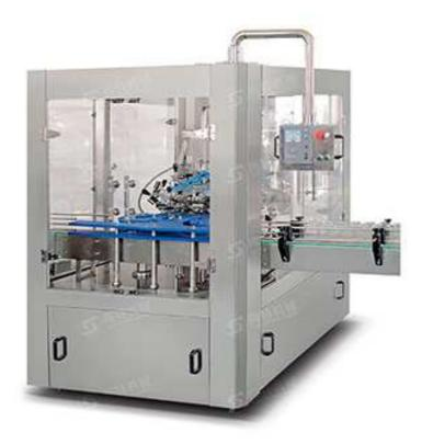
The fully automatic bottle washing machine can automatically working process from bottle entry, bottle rinsing, water removing to sanitized bottle out. The automatic bottle washing machine absorb in high technology from aboard, by adopting gyration method on rinsing device. This equipment is designed to improve efficiency and maximize output while reducing environmental impact.
