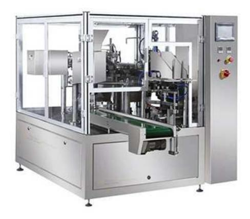
Food feed bag packaging machine is specially used to package granular food. The light signal is converted into electrical signal, controlled by the PLC system, and the photoelectric system is applied to the horizontal premade pouch packing machine. The pneumatic device is used to achieve a very accurate count, 100 per package. The error of the screw is 0, and the error of 1000 per pack is 1. It is a pneumatic device, and the power consumption is 1/200 of the traditional machine.
