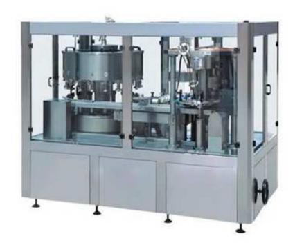
The series equipment is used for filling juice, hot drink, water, etc with PE can or Tin can.
