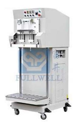
CE-600/DZQ series External Type Vacuum Packing Machine not only can do the process of sealing, but also vacuum extraction or inert gas flushing after vacuum cycle.
