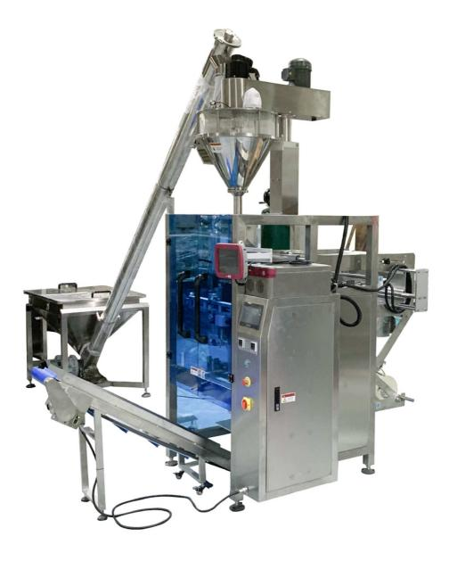
The powder packaging machine with laser coding machine is applied to different powder package; and the laser coding for manufacturing date has a longer storage time and the printing range is also more flexible than common ribbon printer; From the video, the whole set production packaging line has gusset function and pillow function, and air exhaust and dust collection are always necessary for a powder package.
