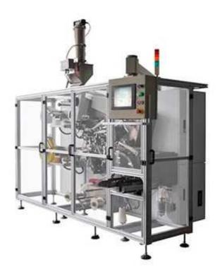
This is our two chamber tea bag packing machine, it makes cold sealing double chamber tea bag automatically, the high speed reach 120 bags/min, also you can connect with our W120 packing machine and make inner and outer tea bag.
