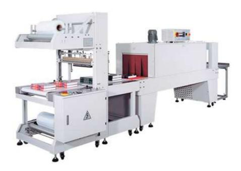
Link-6030A +Link-6040 cuff packing machine is designed for a single object or articles with paper support, this machine and production line docking automatic feeding, wrapping film, sealing and cutting, shrinkage, cooling finalize the design, unmanned flow work.
