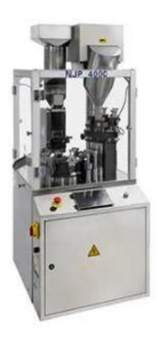
Small Fully-auto capsule filling machine NJP-400C processes the products for optimal productivity up to 400 capsules per minutes, featuring low-maintenance operation, minimal downtime, and overall dependable production. Small automatic capsule filling machine, Small automatic capsule filler machine.
