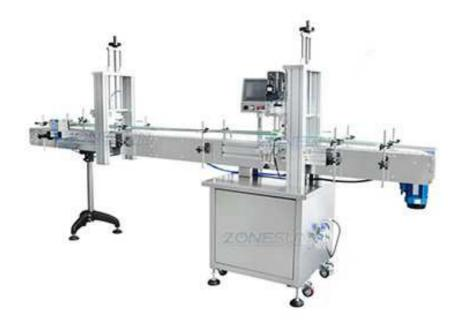
This automatic capping machine has functions of pressing and screwing caps. The pressing head and capping head can be used at the same time or choose one of the two. It is easy to adjust and operate; this machine is widely used in food, beverage, cosmetics and daily chemical industries.
