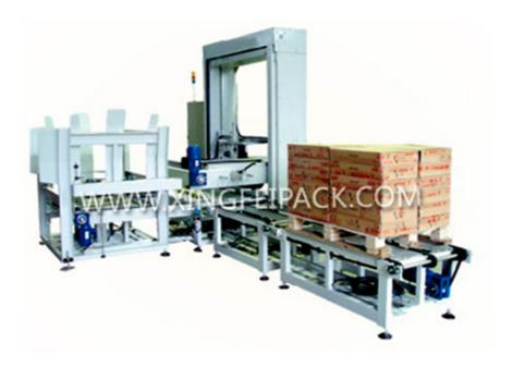
This machine is used for accumulating and stacking the loaded cartons to the pallet automatically, can stack for layers, then sent out of the palletizer, easy for the forklift taking to the warehouse. It is consists of carton feeding and accumulating system, palletized, empty pallet magazine which is widely used in food, beverage, chemistry, pharmacy, wine etc.
