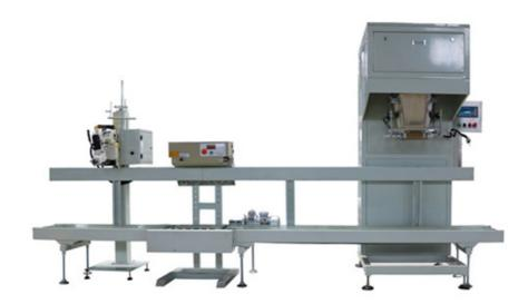
SGJ-Q hopper free weighing bagging machine system adopts hanging weighing system for different kinds of material. The manual bagging machine units shall use instrument panel for machine control & operating which is easy to learn and operate. Now this semi-automatic bagging machine unit is widely applied for granular materials like granular fertilizers, agro-chemicals, animal feeder, raw chemical material, seeds, and rice and sugar industries.
